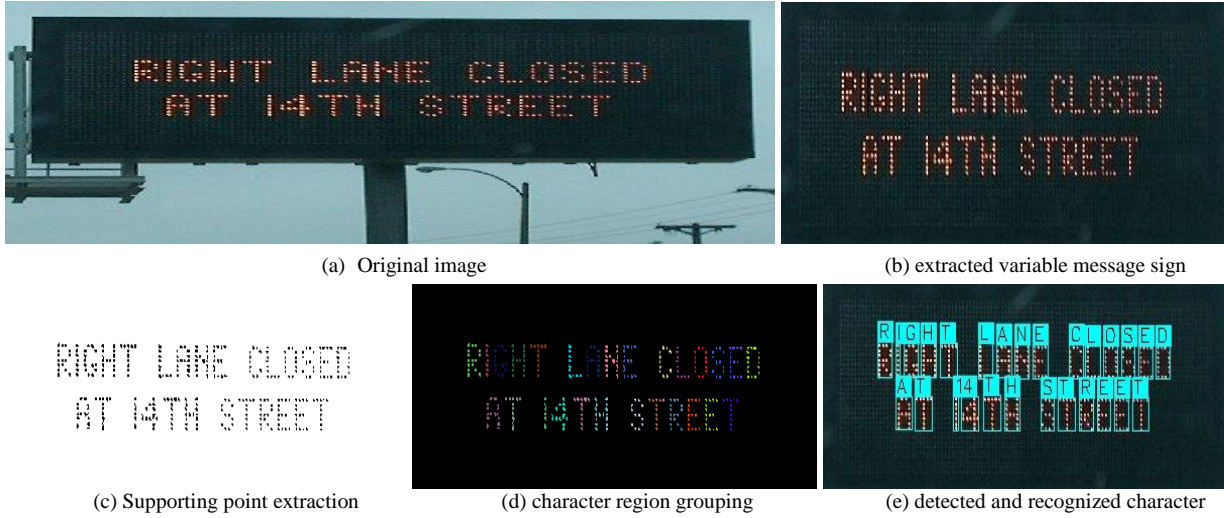
Fig. 2. The illustration of the process of character recognition in variable message sign.
