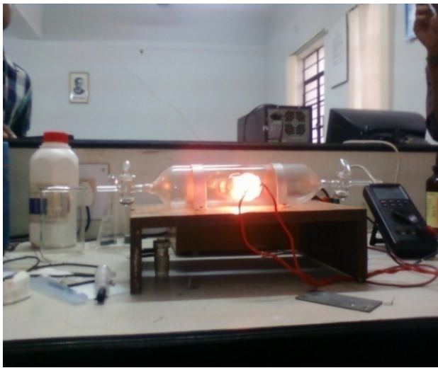
Fig. 1. Zinc Oxide Gas Sensor with heating coil arrangement [1]
